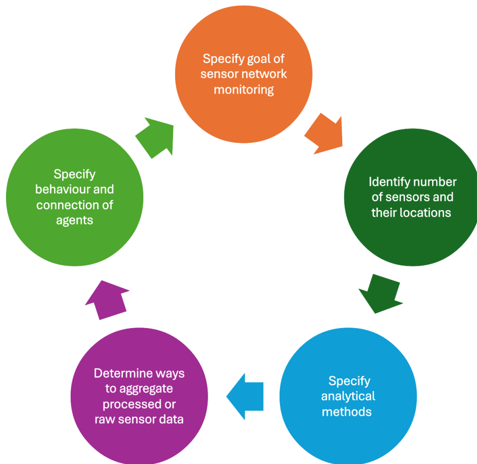
Figure 2. General workflow of modelling agent-based sensor networks
